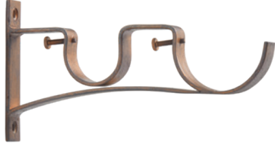
Harlan Double Bracket PO214HADBK 3 3/4" H x 3/4" W backplate, 6" front return and 2 1/2" back return, front cradle holds 2 1/4" DIA pole, back cradle holds 1 3/8" DIA pole Metal, Couture
