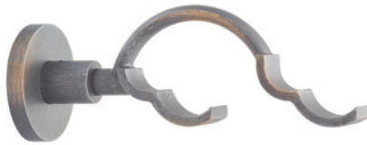
new Talon Double PO138TADBK 2 1/2" DIA backplate, 6 1/2" front return and 3 1/2" back return, 3/8" clearance above backplate, use with Calla C-Rings Metal, Patina
